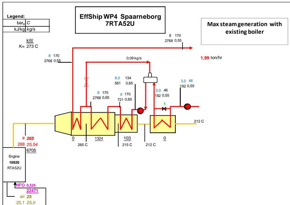
Figure 3 Prevailing performance of existing boiler
