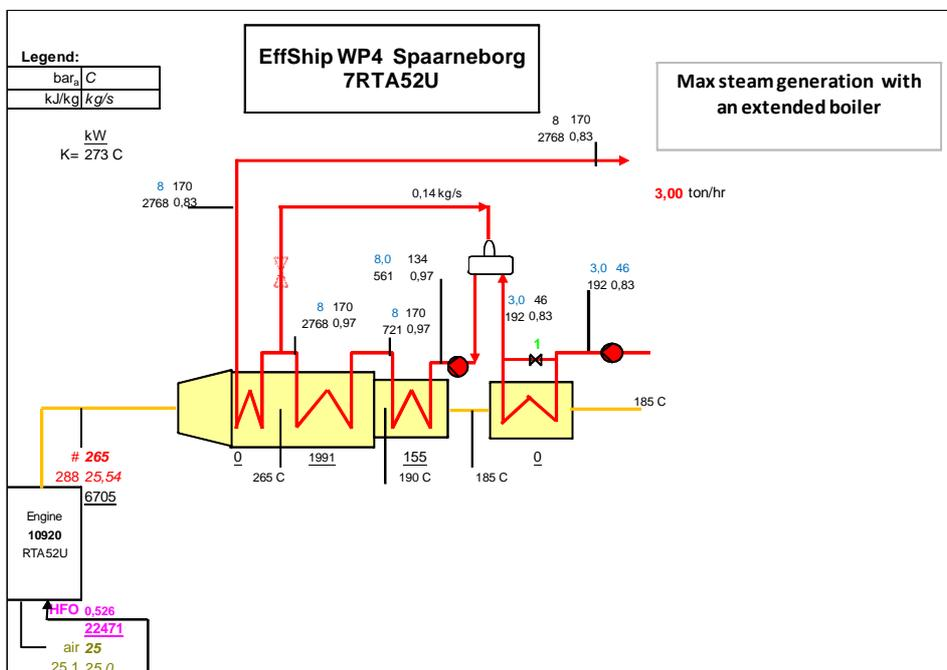
Figure 4 Capacity increase for a modified boiler
