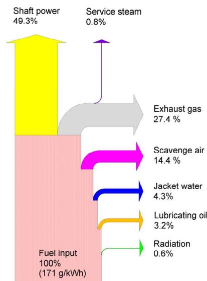
Figure 1 Sankey diagram of a two stroke diesel engine
